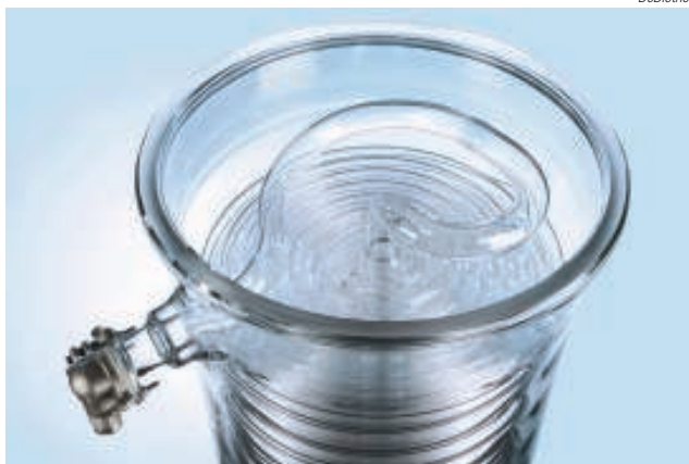
FIGURE 1. QVF coil-type heat exchangers are made of borosilicate glass 3.3 and are single-piece units where the tube coil is fused to the shell, so that no seals are required, which eliminates the risk of cross-contamination between the service medium and the product
