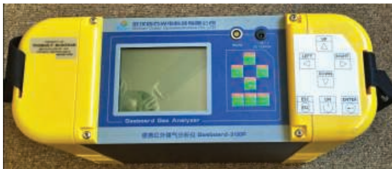
FIGURE 2. More-specialized equipment includes this portable combustion analyzer
